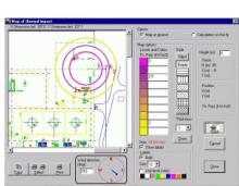
**FLARES** is a software for the correct sizing of **industrial flares** and for the evaluation of their thermal and acoustic impact. All calculations are made according to the **API (American Petroleum Industry) Recommended Practice 521**.
